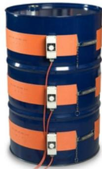
NobleHeat Heater Drum Heaters are an easy way to heat up drum contents. Various sizes and lengths allow you to heat up practically any drum, pail or barrel. Uniform heat prevents scorching or degradation of the contents. The silicone rubber band heater is placed below the level of the fluid. The easy spring lock-up provides movement of the band when content levels fluctuate. The band style drum heater can be used on plastic, alloy or just about any material.
